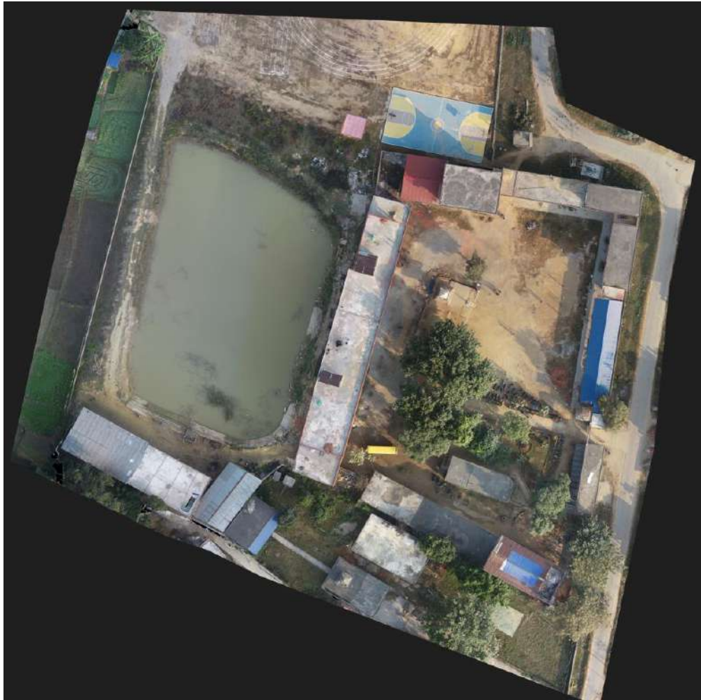
Fig: Orthomosaic of PNSS obtained after processing 222 images.
